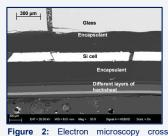
Figure 2. Electron microscopy cross section image of end-of-life c-Si solar panel showing composition and different layers present in solar cell. Chemical composition can be determined by EDX measurements.
